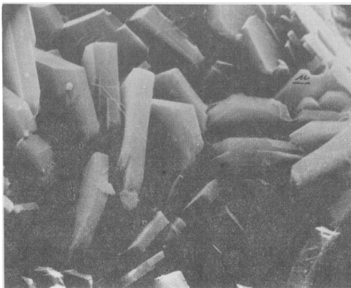
Figure 10. Scanning electron micrograph of clinoptilolite laths with minor amount of mordenite fibers from a lacustrine tuff near Hector, CA. (Mumpton and Ormsby, 1976).
